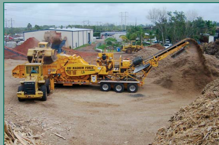
Regrind of Mulch (shows optional overband magnet)
